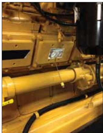
Fig 7. Thermocouple shown attached to the test engine block (above). Temperatures from all points were captured using a temperature data logger (below).
