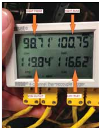
Fig 7. Thermocouple shown attached to the test engine block (above). Temperatures from all points were captured using a temperature data logger (below).
