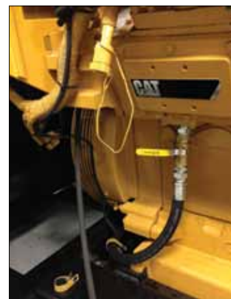
Figure 5. The test engine's left side showing CSM supply port. The supply port is mounted to the opposite side to ensure even heat distribution.
